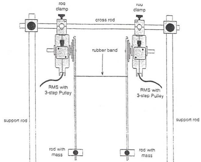
Motion Sensors were attached to Data Studio and used to graph the motion of the rods. The masses were used to change the effective length of the pendulum by moving the center of mass up or down along the rod.
